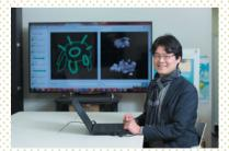
In order to produce a 3D object from a 3D printer, a method is required to make 3D models. This photo shows a system for easily producing 3D models from hand-drawn sketches. If the desired object is drawn in 2D (left-hand side of monitor) the Al will display a 3D representation of what it thinks you are trying to create (right-hand side of monitor). A continued dialog between the human and the Al will lead to the creation of the desired object.
